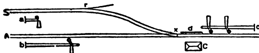
FIG. 5.—Interlocked signals (American practice, signals at right track, and arms at right of post).
