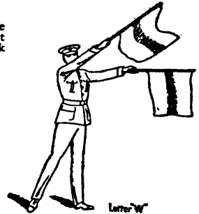
Fig. 3.—Semaphore (the thin upright strokes represent the seaman's body, the thick strokes his arms).
